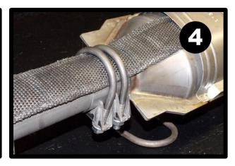
Secure the CatStrap and harden steel pins in place using the included exhaust pipe clamps. Once the clamps are tightened it will provide a per meant and difficult to remove installation.
