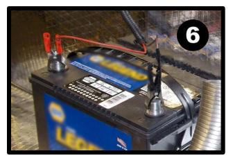
Use included nylon tie and/or Velcro strips to secure the alarm siren inside the engine compartment to any non-heat producing horizontal or vertical object with a circumference of less than 4" within general vicinity of car battery. Electrical battery cables most often serve as an appropriate alternative. DO NOT mount alarm siren with horn facing up. Water can collect in the horn, causing the siren to malfunction. Simply draw hand tight to secure alarm unit to object.
