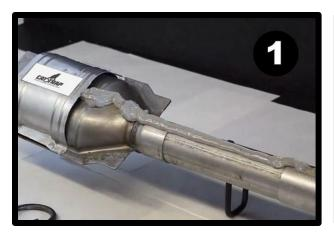
Apply the included bonding paste liberally along the top of the exhaust system.
