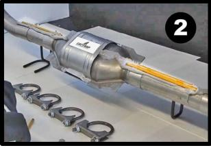
Install the included hardened steel pins at the probable cutting area on top of the bonding paste.
